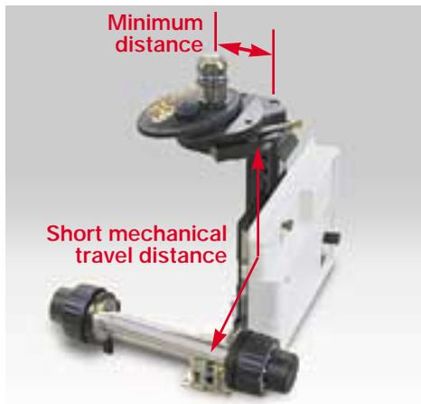
Short mechanical circuit structure and high rigidity nosepiece design avoids pitching and yawing when the nosepiece is manipulated during operations such as DIC prism insertion or adjustment of an objective's correction collar.
