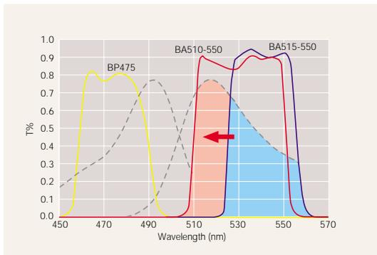
The new IBA cube is optimized to maximize both GFP excitation and detection of GFP emission through the use of a new dichroic mirror with minimal crossover.
