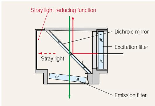
When the fluorescence excitation light is reflected by the dichroic mirror, some light may pass through the mirror and reflect as stray light in the cube assembly. This stray light may reflect out of the cube and into the imaging path, resulting in decreased contrast due to autofluorescence. Low reflection materials are incorporated into the design of all new Olympus fluorescence filter cubes. Such a design absorbs over 99% of all stray light, resulting in high contrast fluorescence images.
