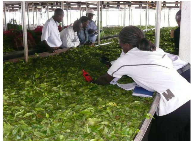
Figure 4: Airflow and humidity measurements during “withering” of tea
