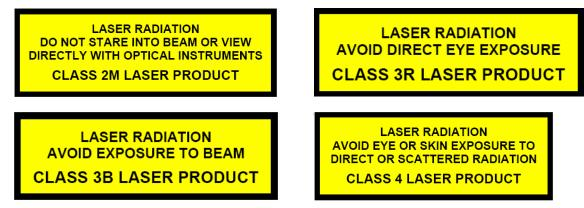
Figure 9-6: Labelling used on laser systems to indicate class and risk.
