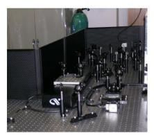
Figure 9-1: Metal barrier with diffuse surface to contain reflections and stray light [16].
