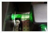
Figure 9-3: High powered laser with an enclosed beam path.
