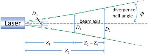
Figure 7-2: Laser beam divergence.
