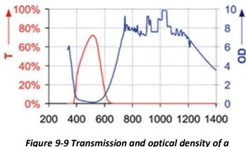
filter used in a set of laser eye protection.
