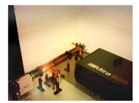
Figure 6-8 Pulsed Ti:sapphire laser system.
