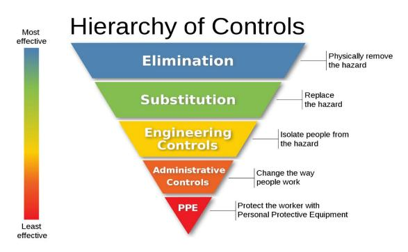
If the laser hazard cannot be removed completely or substituted for a less hazardous then in any given situation engineering controls are paramount. The hierarchy for control measures can be summarised as
