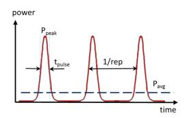
Figure 7-1: Illustration of a laser pulse.
