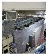
Laser curtains (example in *Figure 9-2*) can be used to completely enclose a Nominal Hazard Zone around a laser. If appropriate, the curtains can be interlocked in the way a laboratory entry point (door) would be. When curtains extend from floor to ceiling safety aspects concerning fire safety, smoke detectors and emergency lighting need to be considered. Laser certified curtains should only be used and the installation should be checked by the RPO.
