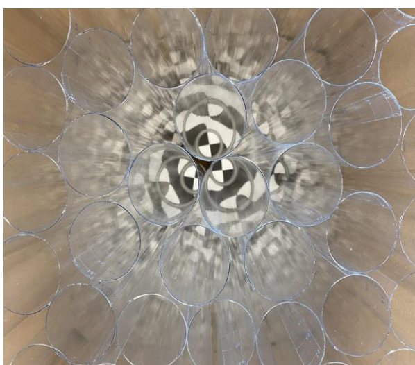
Secchi tubes as part of the Freshwater Watch field sampling kit (picture by @Freshwaterlizzy)
