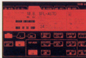
1. Photomicrography conditions setting screen Selection of camera, framing, photomicrography mode and exposure mode can be made via this screen.
