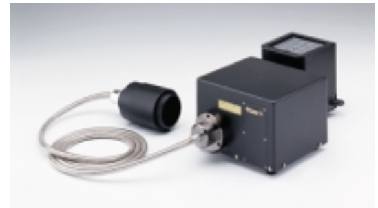
Transmitted light detection module External transmitted light photomultiplier detector and 100W Halogen conventional illumination, integrated for both laser scanning and conventional transmitted light Nomarski DIC observation. Motorized exchange between transmitted light illumination and laser detection. Simultaneous multi-channel confocal fluorescence image and transmitted DIC acquisition enabled.
